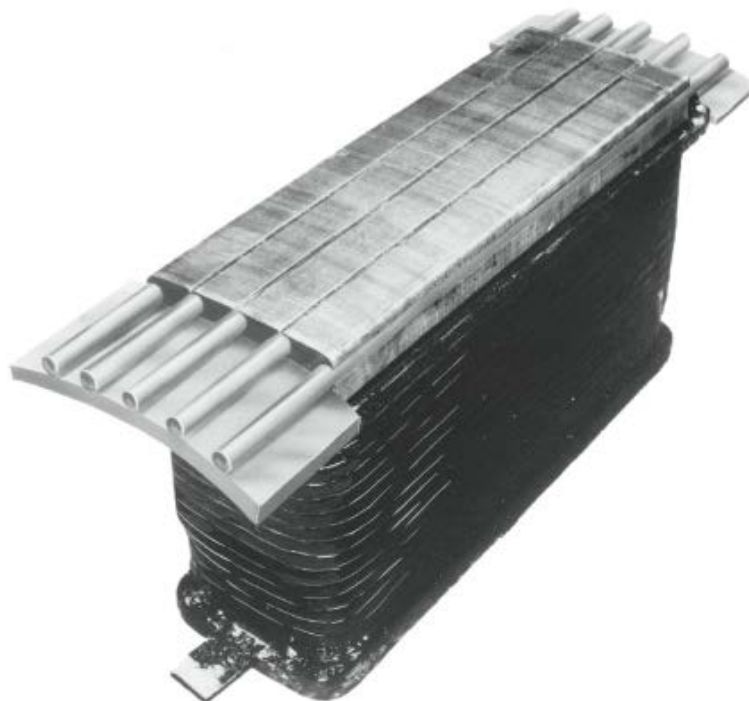
A simplified diagram of a salient two-pole machine showing amortisseur windings.
